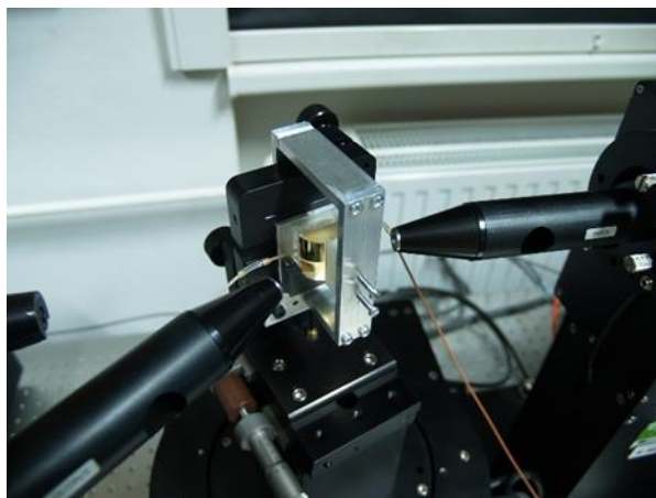
Figure 1: V-VASE based SPR-TIRE instrumentation
