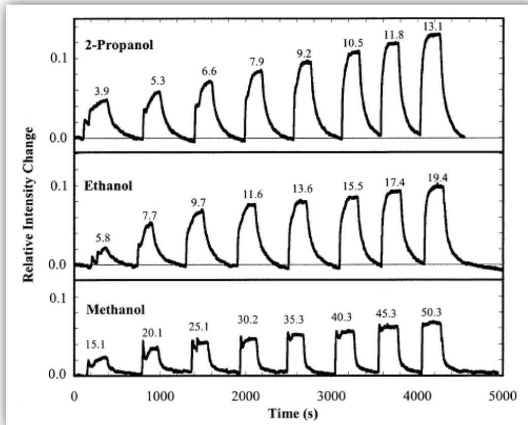
a thermally oxidized porous silicon layer exposed to ppm concentration vapors of 2-propanol, ethanol and methanol
