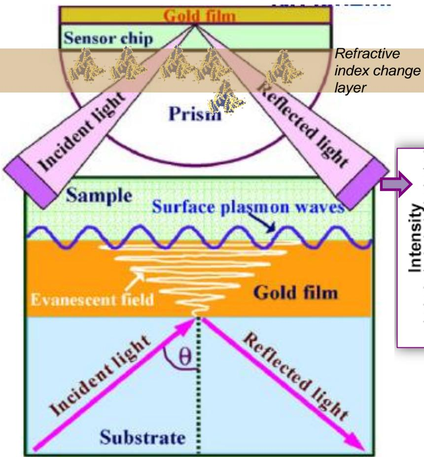
Adsorption of biomolecules (antigen or antibody) or gas on the metallic film as well as molecular interactions (antigen/antibody complex) will induce a change in the refractive index near the surface, thus giving rise to a shift of the resonance angle.
