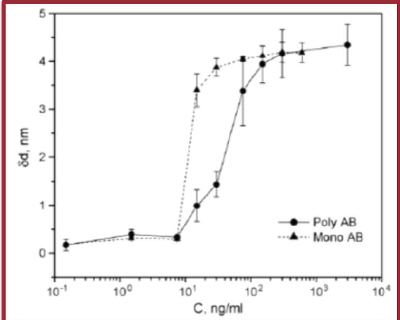
Changes in the adsorption layer thickness caused by T-2 mycotoxin adsorption vs T-2 concentration in solution
