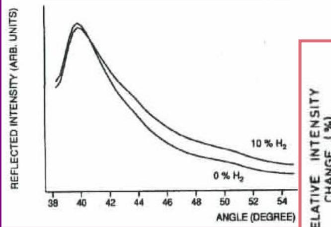
Reflected light intensity vs angle for a 200Å Pd film exposed to H<sub>2</sub>
