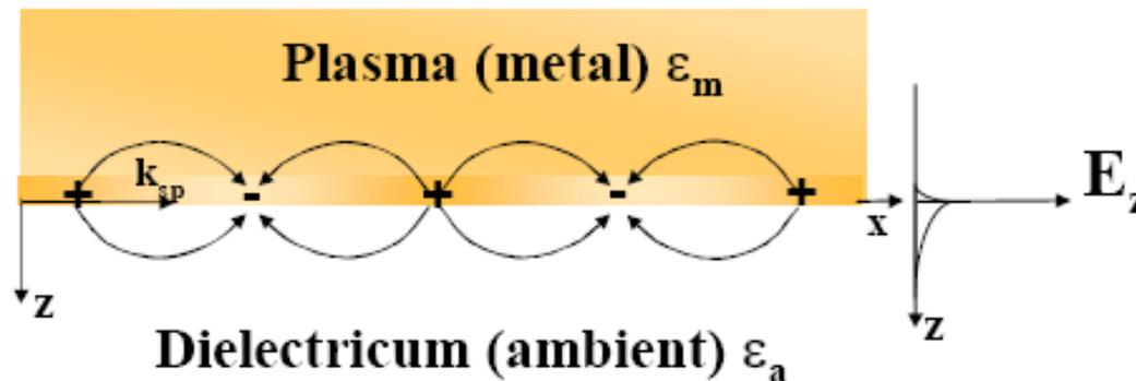
P-polarized surface bound electromagnetic wave.
