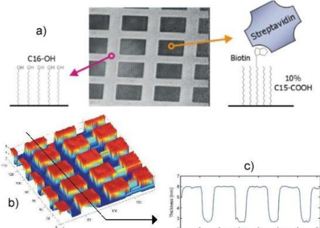
**a)** A gold surface was patterned with two different alkanethiols, biotin was coupled to carboxyle groups in the squares and streptavidin was washed over the surface. The image is taken with imaging ellipsometry and a clear contrast can be seen. **b)** The data in the image is transformed into a thickness map of the surface. **c)** A line profile taken from the thickness-map; the squares are approximately 3 nm higher than the frames.
