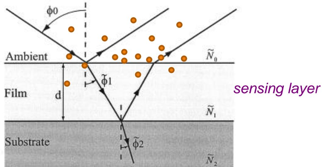
Three-phase model representing a substrate with a sensing layer
