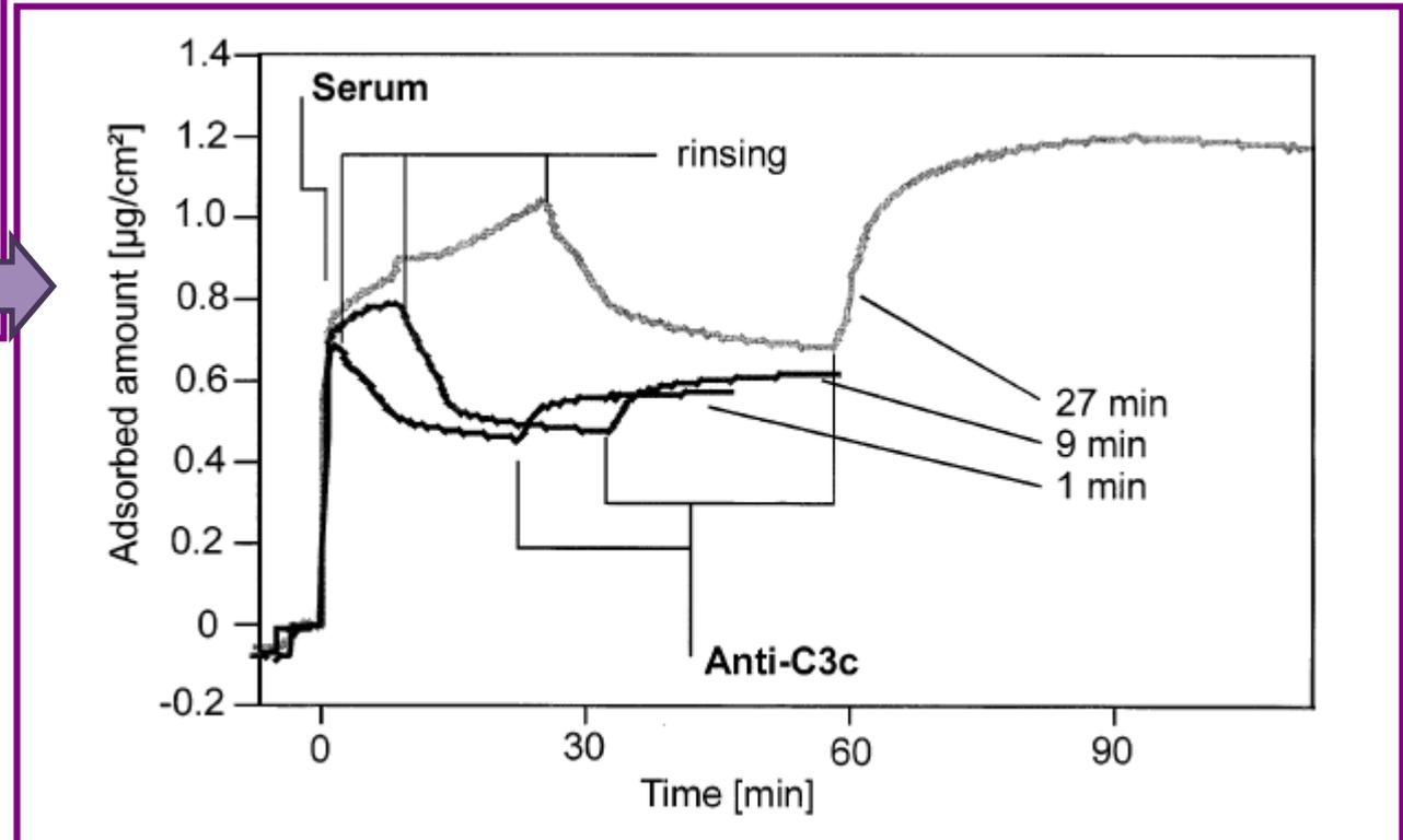
Serum adsorption versus time measured on  $\text{TiO}_2$  followed by rinsing in buffer and subsequent binding of anti-C3c. The three adsorption curves correspond to different serum incubation times: (a) 1 min (b) 9 min and (c) 27 min.
