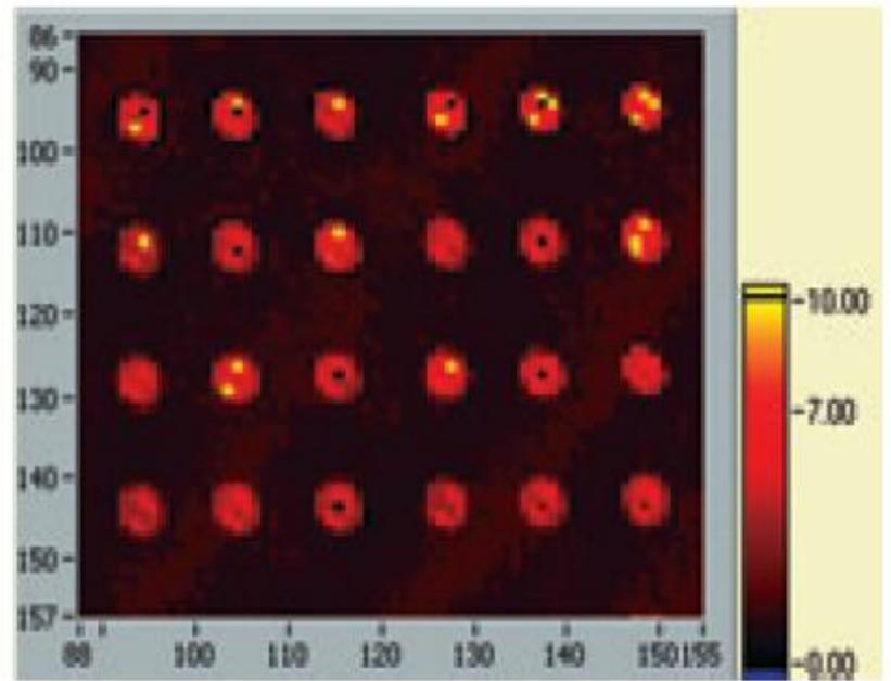
Thickness-map [z in nm and x/y in pixel] of protein array on a gold surface
