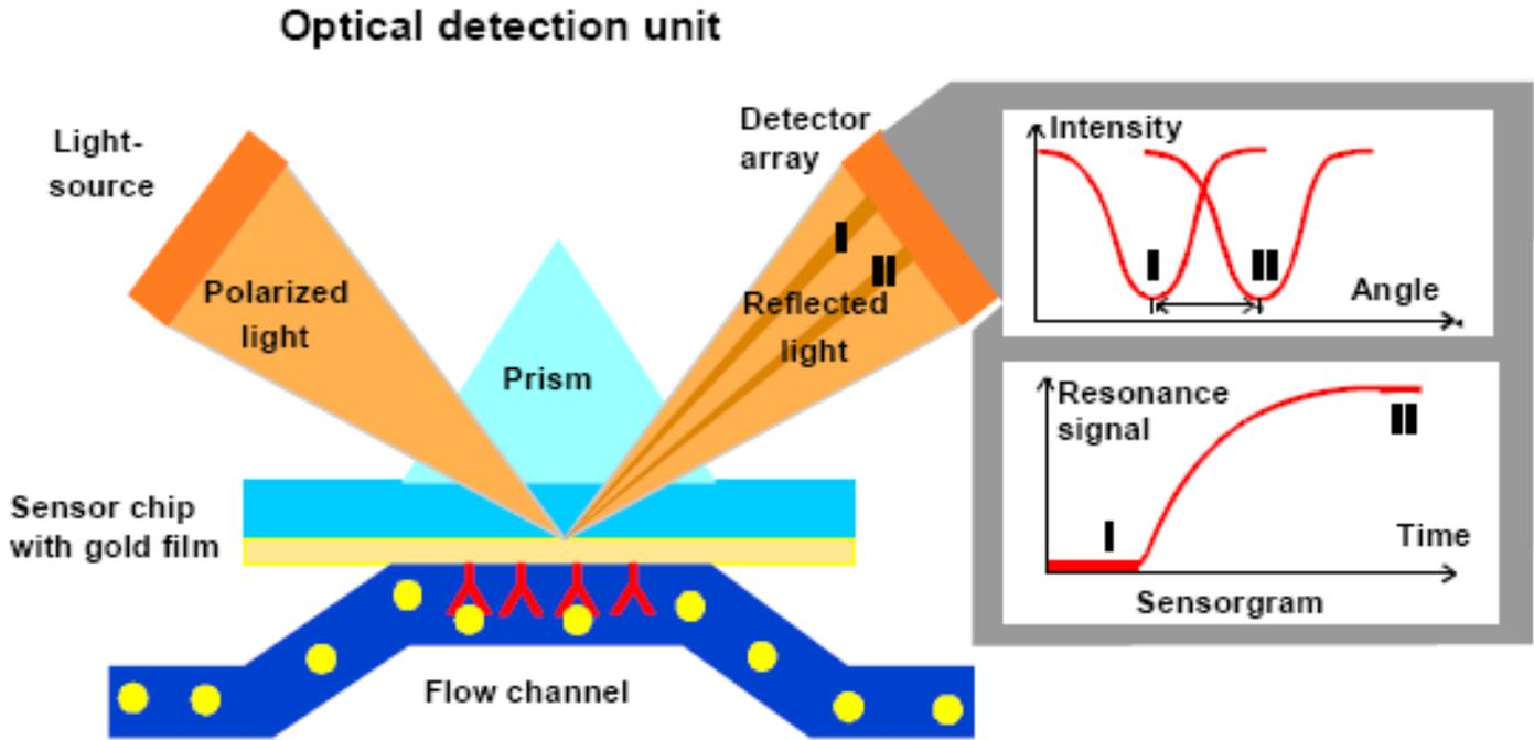
As biomolecular interaction events will lead to an increase in refractive index or thickness of the organic layer adsorbed by the gold sensor surface, which can in turn change the conditions for wave-vector matching, any biomolecular binding reaction taking place in the sensor surface will therefore result in a shift in the SPR dip both in the angular and spectral domains
